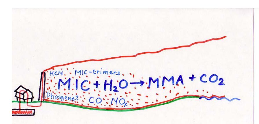
The cloud contained a mixture of substances. Concentrations were higher close to the plant. The gases were heavier than air, displacing oxygen.
